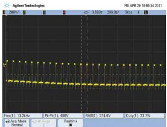
These two scope waveforms are taken at a much higher sweep speed (200us/div) than those overleaf to illustrate the variable pulse width of the synthesised motor waveform. The waveform with the high pulse duty cycle is delivered on positive excursions of the waveform while the low pulse duty cycle is equivalent to the negative duty cycle.
